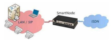
SmartNodes are also widely used to connect to analog PSTN lines or to integrate fax machines and other existing equipment. To make things easy for the end user and system integrator, the 3CX software contains an **integrated SmartNode configuration file generator**. With a few mouse clicks, it generates a full SmartNode configuration file, ready to use and fully interoperable with the system.
